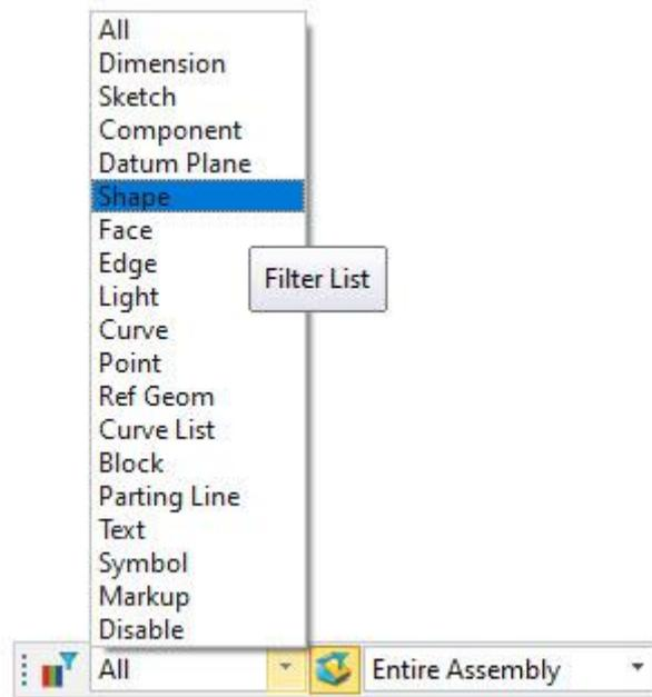
**Holding the Shift key + Right mouse button**, the filter list will display on your mouse pointer position.
