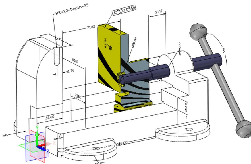
**Note:** To set the different components to different display modes, you can right-click the component >Display>then select your needed display mode.
