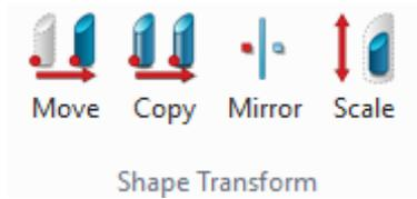
Shape transform commands support to move, copy mirror and scale the selected shapes.
