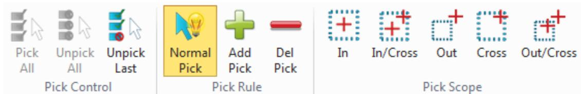
**Pick control:** Control the input field, picking or unpicking. You can also call the pick control by a right mouse button click on the graphic window.
